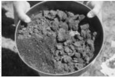
Field demonstration at Northern Illinois Agronomy Center: Aggregates obtained by dry sieving reveal a lot about soil condition. Granular structure (lower left) is more desirable.
